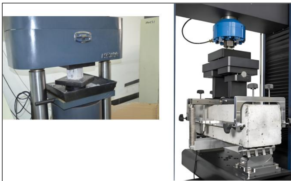
Figure 2. Compressive Strength and Flexural Strength Testing Equipment
