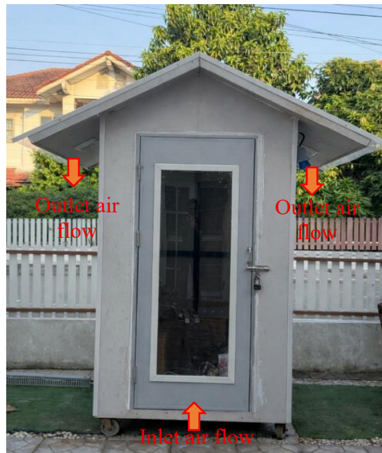
Figure 2 Photograph of the experimental house (House 1) used for data collection in the evaluation of the system's thermal performance.
