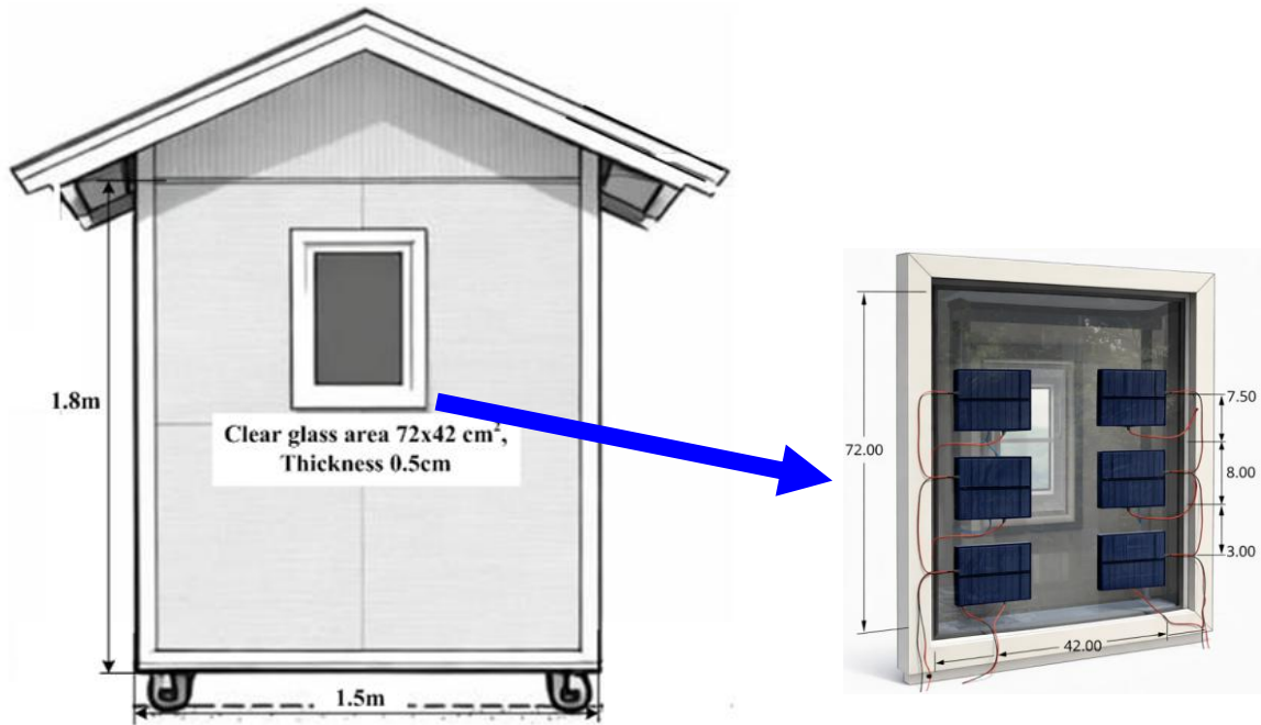
Figure 2 Small-scale house model used for testing the transparent glass window (left) and the transparent glass window integrated with PV cells for electricity generation (right).
