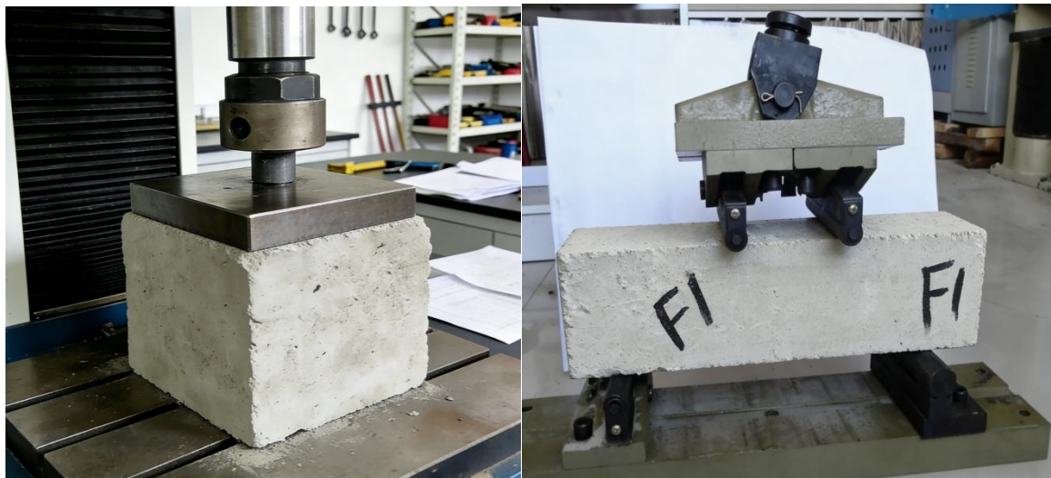
Figure 3 Flexural strength testing setup: (left) prism specimen positioned on the universal testing machine under third-point loading, and (right) close-up of the loading arrangement on the prism specimen.
