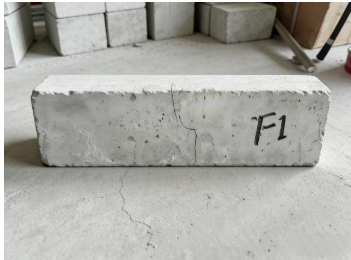
Figure 4 Pre-cracked prism specimen (F1) after controlled third-point loading, showing a visible transverse crack (0.10–0.20 mm) at the mid-span bottom surface.
