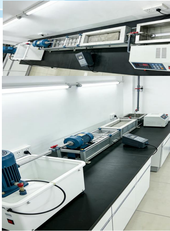
Figure 6 Hydraulic scouring test apparatus used to simulate rainfall runoff effects on pre-cracked specimens at a flow rate of 1 m/s for 72 hours.
