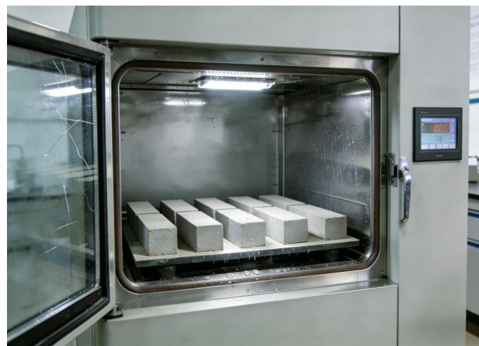
Figure 5 Pre-cracked prism specimens placed inside the environmental chamber for thermal cycling simulation (7 cycles, 40°C/20°C).
