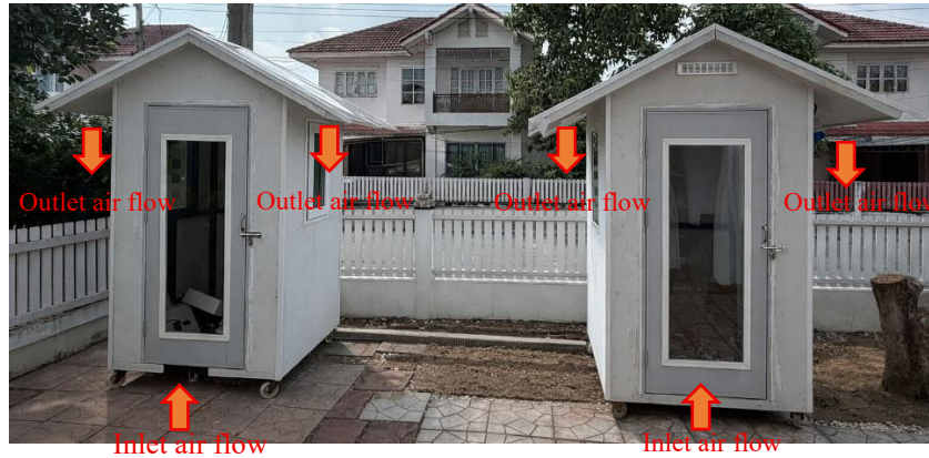
Figure 2 Photograph of the experimental house used for data collection in the evaluation of the system’s thermal performance.
