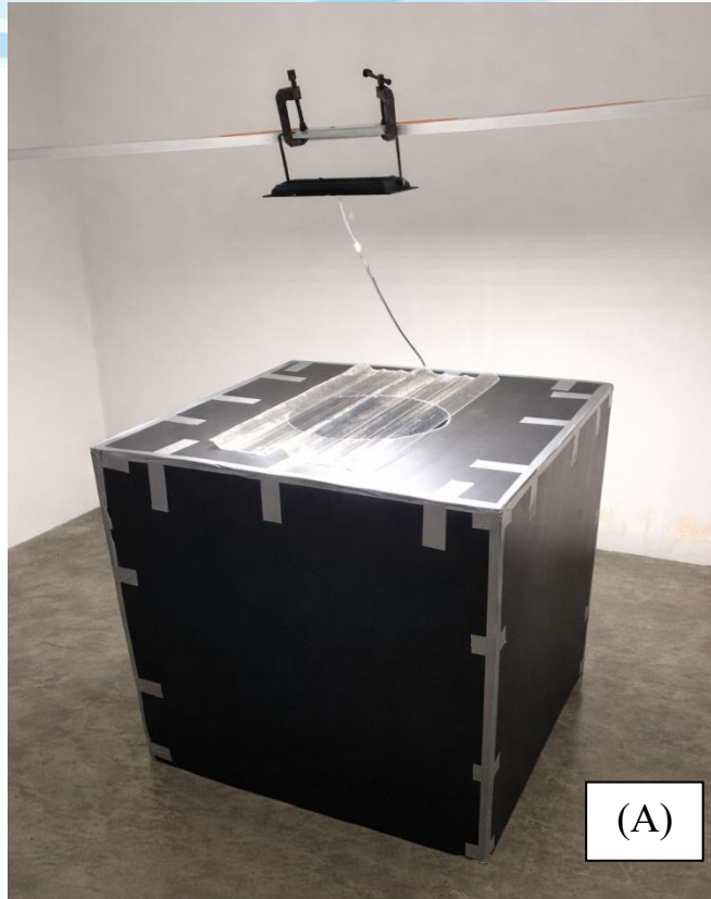
Figure 5. Experimental chamber equipped with clear corrugated polycarbonate roofing panels.
