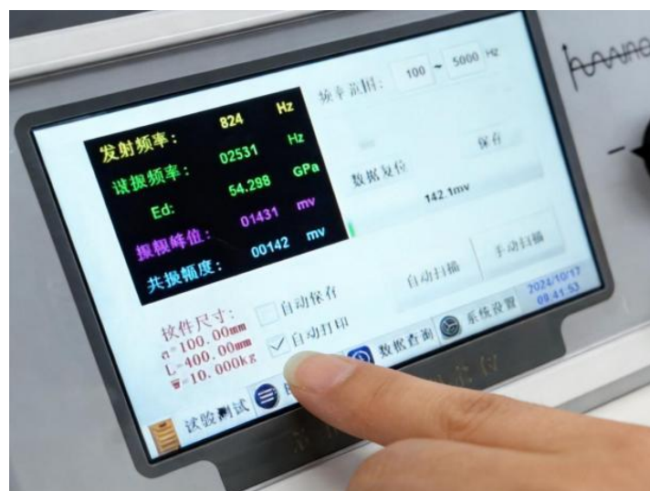
Figure 2. Digital display of the dynamic elastic modulus tester during resonance frequency measurement.
