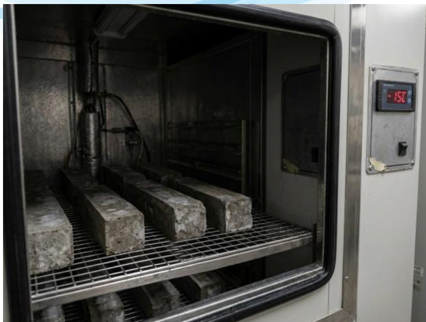
Figure 4. Rapid freeze–thaw testing chamber used for durability assessment of concrete specimens.
