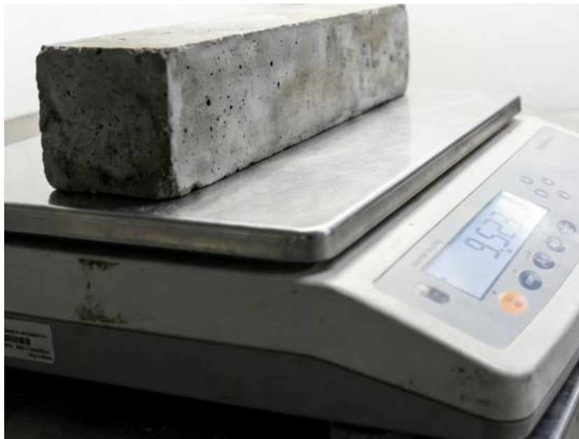
Figure 3. Mass measurement of prism specimen in saturated surface-dry condition using a digital balance.
